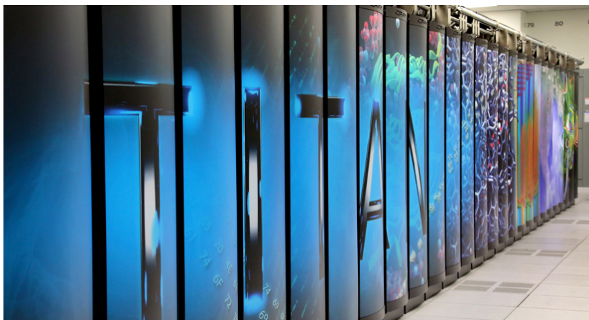
The Titan supercomputer at Oak Ridge National Laboratory near Knoxville, Tenn., is designed to do more than 20,000 trillion calculations per second. That ability is useful in running computer models of complex and dynamic systems, including Earth’s changing climate. Oak Ridge National Laboratory
